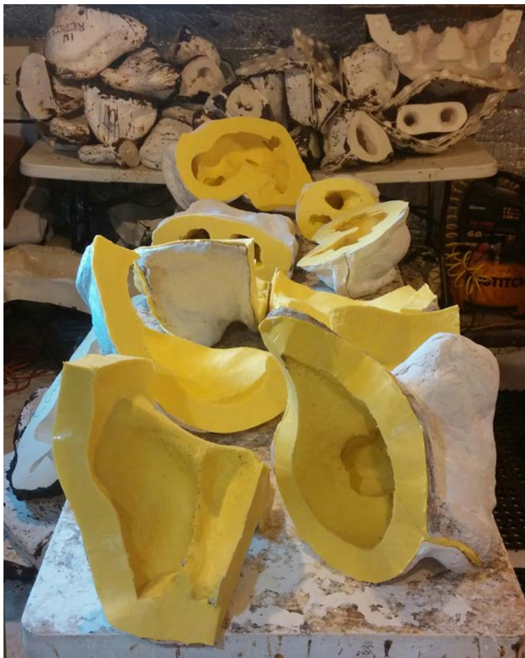
The Merry Sunshine (life-size) mold is ready for wax!
