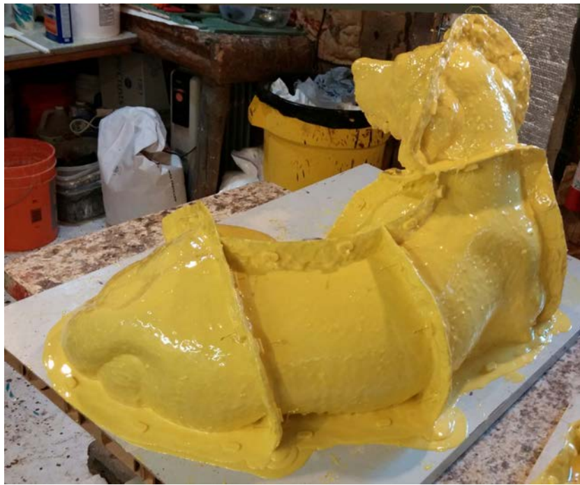
JULY 8, 2015: The mold is shown apart, complete with the plaster mother mold.
