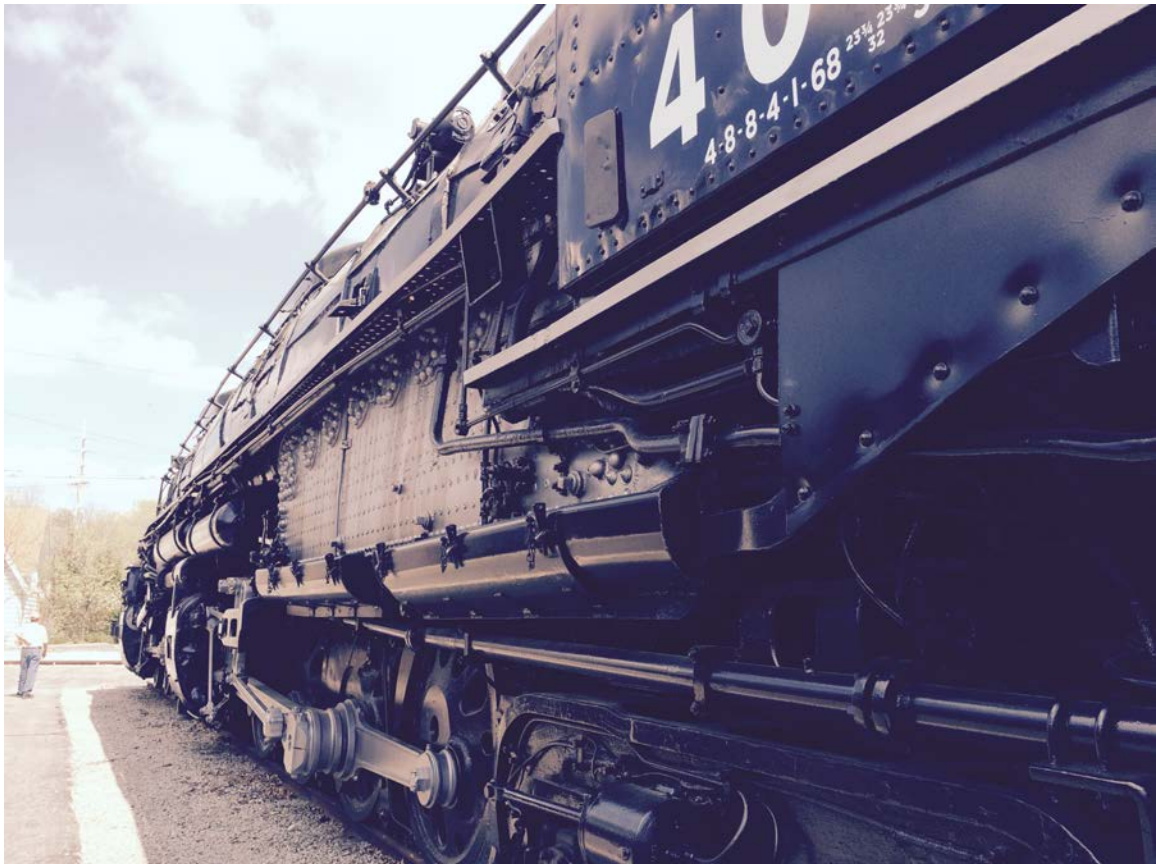
This is the engine room of a Big Boy. I love the mechanics and, of course, the fire pit in the center. From the coal car behind an auger drives the coal up into the fire pit. It's fascinating, at least to me. Big Boy is the popular name of the American Locomotive Company 4000-class 4-8-8-4 articulated, coal-fired, steam locomotives manufactured between 1941 and 1944.
